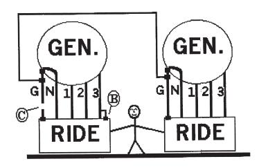
There will be an electrical path from phase three of the generator on the left side - to the left ride which has the fault - through the person touching both rides - to the ride on the right - thru the right ride's "grounding" conductor (green) - to the generator which supplies power to the right ride - thru the bonding conductor between generators - back to the original generator, on the left side.
